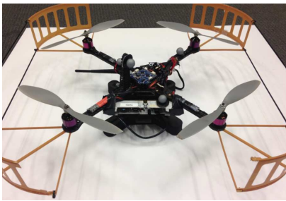
Fig. 16. Asctec Pelican with Primesense RGBD sensor.
